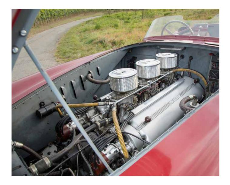
unit). The engine also featured single intake porting versus the Colombo V-12's siamesed arrangement, and twin ignition per cylinder for increased power.
