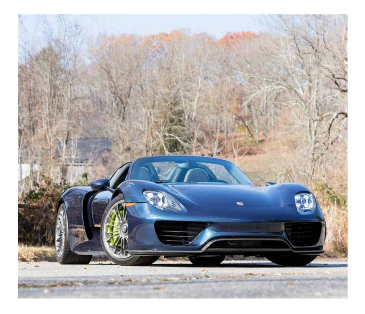
at low speeds and increased stability at high speeds. With electric motors at both axles, the car was able to recover energy which was normally lost at braking to recharge its own batteries. Like the Carrera GT, the roof can be fully removed so one can experience the 918 as a coupe or in the style of a targa.
